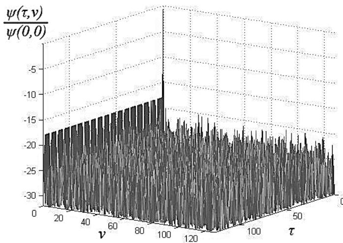
Figure 3. AF of synthesized sequence with length  $N=511$
